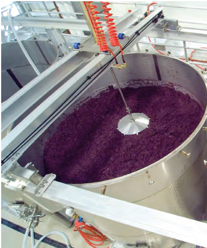
A pneumatic punchdown device is used to manage caps in the open-top tanks.
