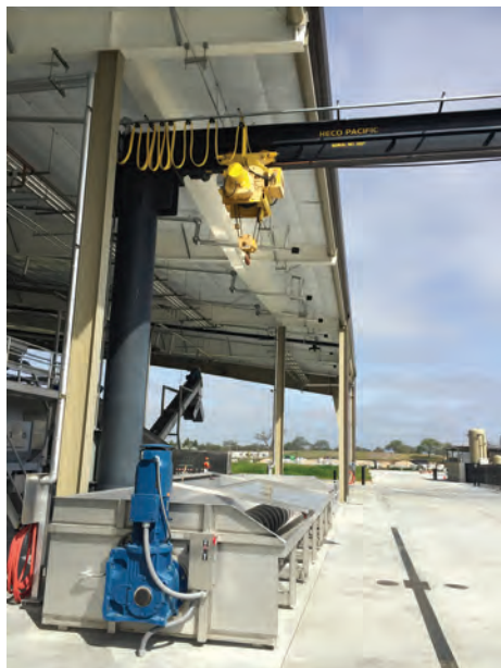
A large crane and auger are used for the largest grape deliveries to the winery.
